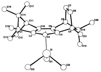
Fig. 1. A view of the molecular geometry of "(+)-(diborna-Cp)ZrCl<sub>3</sub>" (7a). Selected bond lengths (Å) and angles (deg): Zr-Cl(1) 2.358(1), Zr-Cl(2) 2.377(1), Zr-Cl(3) 2.372(1), Zr-C(2) 2.506(2), Zr-C(3) 2.453(3), Zr-C(4) 2.447(3), Zr-C(9) 2.577(3), Zr-C(10) 2.609(3), C(2)-C(3) 1.420(4), C(2)-C(10) 1.420(4), C(3)-C(4) 1.425(4), C(4)-C(9) 1.428(4), C(9)-C(10) 1.407(3), Cl(3)-Zr-Cl(2) 93.2(1), Cl(3)-Zr-Cl(1) 103.3(1), Cl(2)-Zr-Cl(1) 111.2(1). For additional structural data see Table 1.
